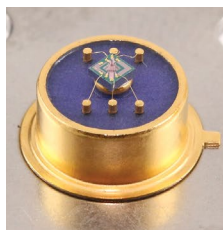
The independently developed MEMS sensor for gas flow measurement (micro flow sensor) Size 1.7×1.7×0.5mm
